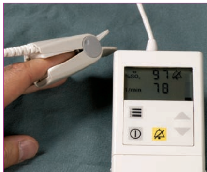
above: A pulse oximeter is useful for measuring the percentage of arterial haemoglobin that is oxygenated.
